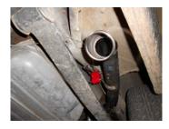
2) Place the right tailpipe **#86191S** over the rear axle so that the rear of the tailpipe exits between the quarter panel and the leaf spring. Repeat this step for the left tailpipe **#86192S**. Connect the hangers on the tailpipes to the rubber mounts installed in the previous step.
