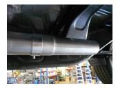
2) If installing the system on a Crew Cab truck with a 6.5' bed, place extension pipe **#TB700S** onto the back of the **#26401S** inlet pipe, place a provided clamp onto the slip-fit and tighten enough to hold in position. The extension pipe will not be used on Double Cab-6.5' bed or Crew Cab-5.5' bed models.
