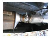
1) Place inlet pipe assembly **#26401S** into position onto the ball connection behind the catalytic converter. Reinstall the clamp onto the ball connection and tighten enough to hold, but still allow for a small amount of adjustment. Connect the hanger on the pipe to the rubber mount on the vehicle.
