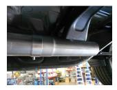
2) If installing the system on a Crew Cab truck with a 6.5' bed, place extension pipe **#TB700S** onto the back of the **#26401S** inlet pipe, place a provided clamp onto the slip-fit and tighten enough to hold in position. This extension pipe will not be used on Double Cab or Crew Cab-5.5' bed models.
