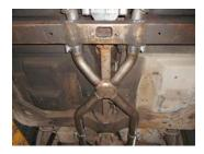
1) After installing the above mentioned downpipe kits or piping to just behind the cross-member, place a provided 2.25" clamp onto the expanded ends of X-pipe assembly **86171S**, then slide onto the back of the manifold pipes (be sure that the pipes are fully slid together). Place a stand under the rear of the assembly and tighten the clamps enough to hold, but still allow for adjustment.
