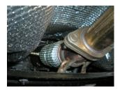
3) In front of the large center muffler, remove the two nuts at the flanged connection just behind the flex joint. Then remove the two bolts from the steel body brace behind the large muffler. Once unbolted, remove the hanger on this section from the rubber mount on the vehicle and lower from the vehicle and set aside. Save the gasket from between the two flanges for use with the Flowmaster system.
