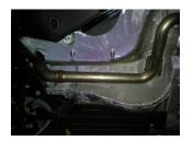
2) To remove the factory exhaust system you will have to cut the system in half. Cutting just before the pipe goes over the rear axle system will allow both halves of the system to be removed easily. After cutting, support the rear muffler with a stand and remove the three hangers on this section from their rubber mounts. You can now lower this section from the vehicle. This section may take some turning and twisting to get the pipe over the rear axle.
