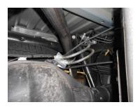
Place left front tailpipe section **#86094S** into position over the rear axle and slide into the left muffler outlet. Place a supplied 2-1/2" clamp onto the back of the pipe. Place left rear tailpipe section **#86404S** onto the front section, and connect the hanger welded to the rear of the pipe into the rubber hanger installed in step 3 above. Pipe should be centered between the shock and the spare tire when adjusted. Tighten the clamps just enough to hold in position.
