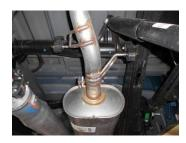
2) Support the muffler with a stand. Using a hacksaw or sawsall, cut the stock tailpipe off just behind the muffler. Separate the wire hangers on the tailpipe from the rubber mounts on the vehicle and remove the tailpipe from the vehicle. This step is not mandatory but makes removal easier.
