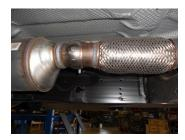
3) Using a 15mm wrench, loosen the bolt on the clamped ball connection behind the catalytic converter. Separate the wire hangers from the rubber mounts on the vehicle and lower the inlet pipe and muffler from the vehicle. A lubricant will make removal much easier. You will need to remove the ball clamp from the stock system; it will be reused with the Flowmaster system.
