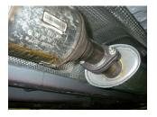
4) Support the large center muffler with a stand and remove the two nuts at the flanged connection just behind the catalytic converter. Once unbolted, you can now lower the front of the system from the vehicle.
