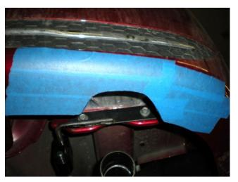
4) Use a jigsaw, sawsall or die grinder to carefully cut along the contour. Use a file to clean up the edges after cutting.
