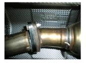
5) Using the 5/16" bolts, nuts and washers provided, bolt inlet pipe **#16745S** to the back of the catalytic converter flange. Using two of the supplied **HA168** rubber hangers, remove and replace the two factory rubber mounts just behind the rear axle. The new rubber hangers will provide much better support to the new Flowmaster system. See Figure A and B in step 10 below for how the **HA168** hanger should be placed onto the factory hangers.
