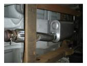
5) Place the provided 3" clamp onto the inlet of muffler #8530562-Z, then connect the inlet of the muffler to the inlet pipe and support with a stand. Tighten the clamp just enough to hold in position.
