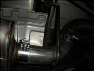
6) Take tailpipe **#26348S** and place it into position over the rear axle. Slide the two hangers on the pipe into the stock hanger mounts on the vehicle. Then slide the front of the tailpipe into the outlet of the muffler. Tighten the clamp enough to hold, but still allow for adjustment.
