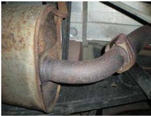
1) To make the removal of the stock system easier, unbolt tailpipe at the flanged connection at the rear of the muffler. Slide the tailpipe backwards to remove it from the muffler and then forward to remove from the rear rubber hanger.
