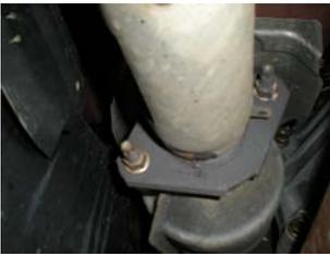
2) Support the muffler with a stand and unbolt the flanged connections behind the catalytic converters. (Save the nuts, bolts and metal gaskets for the installation.) It will be necessary to take a 12mm socket and unbolt the hanger bracket from the frame that holds the head pipe and muffler assembly up (save bracket and bolts, you will reinstall with new system). Remove muffler and set aside.
