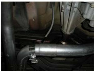
3) Take the left head pipe assembly **#16478S** and right head pipe assembly **#16473S** and slide them together (make sure you slide a clamp on pipes before sliding the two together). Lift the assembly up and bolt the flanges together (make sure you put the metal gaskets between the flanges first) using the stock nuts and bolts. Tighten the clamp on the slip-fit connection just enough to hold in position.
