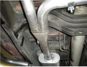
5) Take a 3" clamp and slide it on the inlet of the muffler. Slide muffler inlet onto the back of the head pipe assembly and temporarily support with a stand. Tighten clamp down just enough to hold in position, but still allow for adjustment. Install a 3" clamp onto the muffler outlet.
