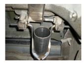
4) Connect the two hangers at the rear of inlet pipe **#16695S** to the rubber mounts on the vehicle and support the front of the pipe with a stand.
