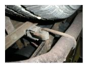
3) Support the muffler with a stand and remove the two hangers on the muffler from the rubber mounts on the vehicle. Lower the muffler assembly from the vehicle.
