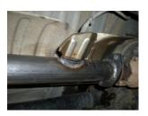
4) Connect the flange on inlet pipe **#16709S** to the flange behind the catalytic converter. Be sure to replace the gasket between the two flanges. Use the included 3/8" bolts, nuts and washers to secure the two flanges together. Use the included 5/16" x 3/4" bolts and lock washers to re-install the O2 sensor to the inlet pipe.
