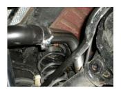
5) Place a provided clamp onto the slip-fit of muffler assembly **#852558-189** and slide onto the back of over-axle pipe **#16669S**. Support the muffler with a stand and connect the hanger on the pipe to the rubber mount of the vehicle. Tighten the clamp enough to hold but still allow for adjustment.
