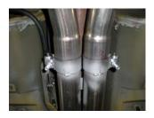
6) Place a 2½" clamp onto the slip-fit of over-axle pipe **#16679S** and slide onto the back of the right Scavenger outlet and support with a stand. Repeat this step with the left over-axle pipe **#16680S**.
