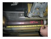
3) To <u>install the new Flowmaster Scavenger X-pipe assembly</u> **#16676S**, the factory Y-pipe must be removed. To do this, measure back 14.00" from the weld at the rear of each of the catalytic converters and make a mark on both pipes. Be sure to double check that the measurements are correct and cut both pipes on the marks. Remove any burrs.
