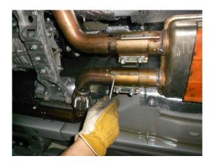
2) Loosen the four nuts at the two band clamp connections just behind the H-pipe in the center of the vehicle. Using a screwdriver, pry up the clips on the clamp body to release the clip from the tab on the inlet pipes. Slide the clamp assemblies slightly back to clear the tabs. With the help of an assistant, slide the over-axle pipes and mufflers toward the rear of the vehicle to disengage from the inlet pipes. Support the rear sections with a stand to allow them to temporarily hang in place.
