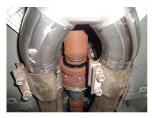
2) Place the factory intermediate pipes with the clamps in place onto the back of the new Flowmaster Scavenger X-pipe and slide the pipes fully together. Center the clamps on the connections and tighten enough to hold in place.
