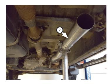
10. Remove muffler hanger mount, slide it onto muffler (3) and place clamp (5) onto muffler. Connect muffler to inlet/extension then fasten hanger mount into place on frame. Tighten clamp just enough to hold parts.
