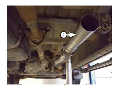
10. Place clamp onto **muffler (3)** then connect it to inlet/ extension while inserting hangers into isolators. Tighten clamp just enough to hold parts.
