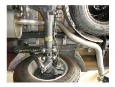
4. Remove (x2) bolts at front flange connection. Slide exhaust system back to disengage hangers from isolators then remove it completely from vehicle.
