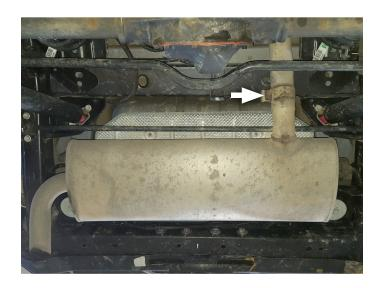
4. Loosen clamp from resonator inlet, disassemble hanger wires from isolators and remove resonator section from vehicle.
