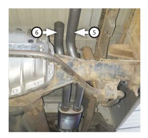
16. Place clamp (14) onto left rear tailpipe (4) then connect it to left front tailpipe. Insert wire hanger into rubber hanger then tighten clamp just enough to allow for later adjustment.
