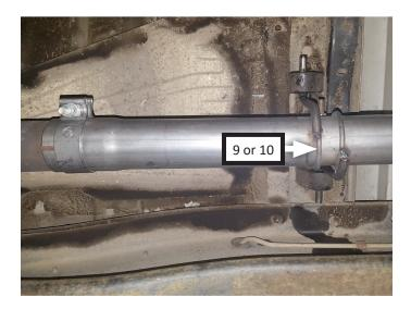
11. Place clamp (14) onto adapter pipe (1) then connect it to extension or factory exhaust. Tighten clamp just enough to allow for later adjustment.
