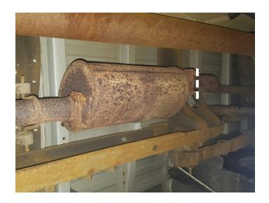
4. Separate wire hangers from isolators behind muffler. Remove bolt and hanger connecting stock tailpipe to vehicle frame (as shown, depending on your application). Remove tailpipe section from vehicle.
