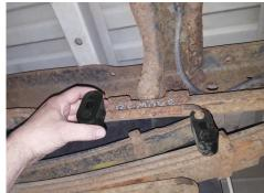
5. Remove clamp on muffler inlet, then remove muffler and set aside.
