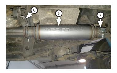
10. Route **tailpipe (4)** over axle then connect it to muffler. Insert wire hangers into isolators then tighten clamp just enough to allow for adjustment.
