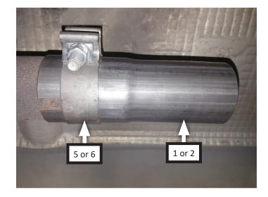
Place clamp (6) onto muffler (3) then connect it to adapter pipe, oriented as shown. Tighten clamp just enough to allow for later adjustment then place another clamp (6) onto muffler outlet.
