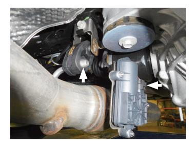
5. Slide (x3) hangers on each tailpipe out of rubber isolators on vehicle and unclip grounding strap from rear hanger on right side of vehicle. With help, remove exhaust system and set it aside.
