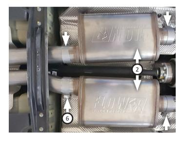
13. Route right (3) and left (4) tailpipes over axle and connect them to mufflers. Insert wire hangers into isolators and adjust tailpipes until tips are level and centered in cut-outs. Tighten clamps just enough to allow for adjustment.
