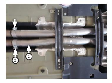
12. Place (x2 ea.) clamps (6) onto mufflers (2) then connect them to scavenger pipe. Level and center mufflers then tighten clamps just enough to allow for adjustment. Place (x2) clamps (6) onto muffler outlets.
