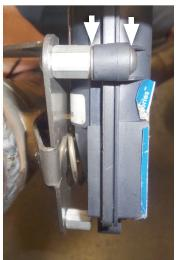
**NOTE:** Check diagram for orientation of scavenger pipe. Once installed, Flowmaster logo must face ground.
