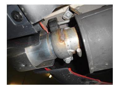
6. Remove (x3) nuts securing actuator to mounts on tailpipes. Remove actuator and spring from mount on each tailpipe.
