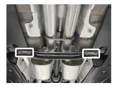
4. Just forward of rear differential on either side of tailpipes, unplug wire from both exhaust valve actuators and tuck them away for later reconnection.
