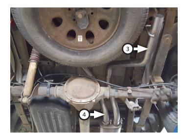
14. Place **clamp (10)** onto **left rear tailpipe (5)** then connect it to left front tailpipe. Insert wire hanger into rubber hanger then tighten clamp just enough to allow for later adjustment.
