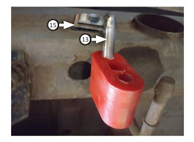
Route right tailpipes (3) and left front (4) over axle then connect them to muffler. Insert wire hanger into rubber hanger then tighten clamps just enough to allow for adjustment.
