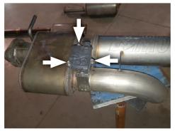
Fasten muffler flange to factory flange using bolts (x2) (10), flat washers (x4) (11), lock washers (x2) (12) and nuts (x2) (14). Secure rear of muffler to exhaust using clamp (7). Re-connect grounding wire.
