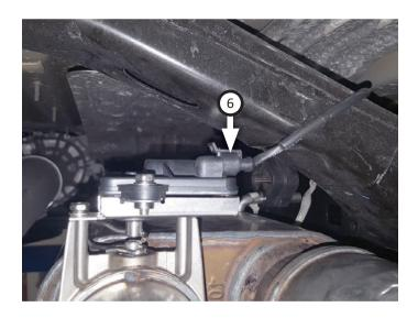
**NOTE:** You may secure wire assembly several different ways; **zip tie (15)** it to factory wire bundle, tuck it behind heat shield, secure it to frame, etc. Just be sure that connections are stable and wire is protected from heat.
