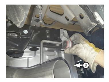
10. Place **tip (4)** onto tailpipe and tighten inlet. Rotate tailpipe and tip to desired distance from body or bumper, so angle cut on tip is properly positioned.
