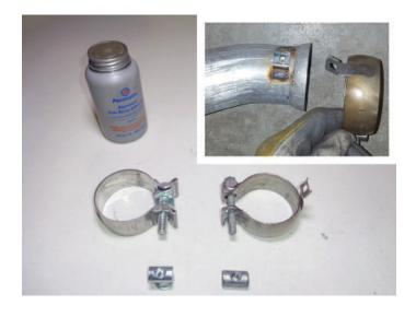
7. Place factory ball clamp (removed step 5) onto **muffler assembly (1)** then connect it to cat. converter. Tighten clamp enough to allow for adjustment.
