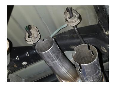
12. Place clamps (x2) (9) onto direct fit muffler outlets then connect factory tailpipes to them. Adjust muffler and exhaust system until it is oriented correctly then tighten all clamps just enough for later adjustment.
