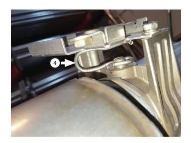
9. Set actuator motor (5) into actuator mount assembly, letting valve spring rest in notch. Fasten components together using screw assemblies (x3) (11).
