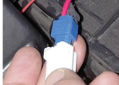
21. Open fuse holder cap, plug in **micro fuse (17)**, then replace cap.
