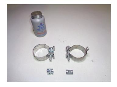
Place 2½" clamp (MC225BS) onto inlet and 2½" clamp (MC250BS) onto outlet of muffler (71416-530) then connect it to factory exhaust outlet. Tighten front clamp just enough to allow for adjustment.
