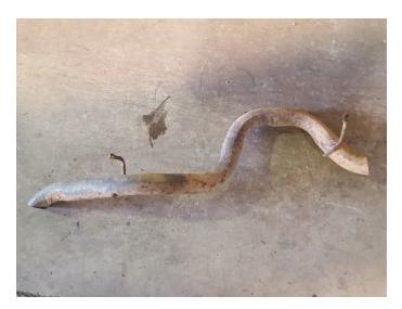
5. Remove clamp and disassemble muffler from catalytic converter then remove muffler from vehicle.
