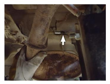
4. Cut tailpipe just behind factory muffler then remove completely from vehicle.
