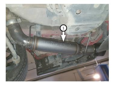
Place clamp (removed step 3) onto left muffler assembly (2) then connect it to left exhaust outlet. Insert wire hangers into isolators and tighten clamp just enough to allow for later adjustment.
