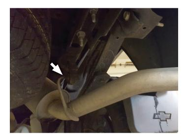
4. Loosen clamp, disconnect inlet pipe at catalytic converter then remove wire hanger from isolator to remove exhaust system completely from vehicle.
