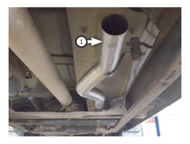
8. Place **clamp (7)** onto **muffler (2)** then connect it to inlet pipe. Tighten clamp just enough to allow for adjustment.
