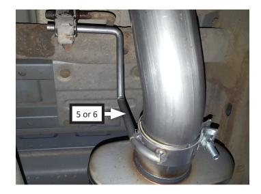
11. Fasten right frame hanger (8) to vehicle using bolt (11), backing plates (x2) (10), flat washer (13), lock washer (14) and nut (12) as shown. Then hang rubber hanger (9) on frame hanger end.
