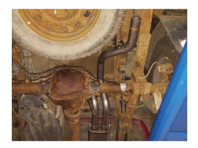
Secure rear frame mount (14) to vehicle using bolt (18) through frame, mount, flat washer (15), lock washer (16) and nut (17). Fit rubber hanger (13) onto end of hanger.
