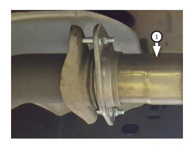
10. For applicable vehicles, place clamp (11) onto extension pipe (2) and connect it to inlet. Inlet pipe should be offset toward frame of vehicle.
