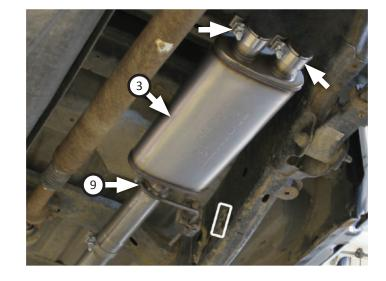
12. Route **left front (4)** and **right tailpipes (5)** over axle and connect them to muffler. Hang wire hangers into isolators and tighten clamps (x2) to allow for later adjustment.
