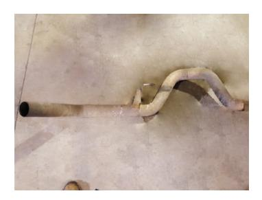
5. Remove bolts (x2) from flange at catalytic converter, disassemble wire hangers from isolators and remove muffler assembly from vehicle.
