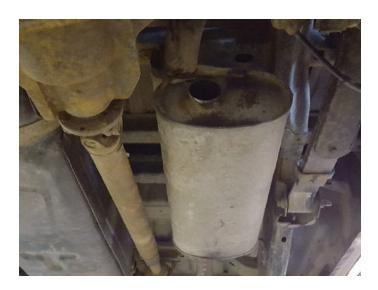
4. Dismount hanger from isolator and remove rear tailpipe section.
