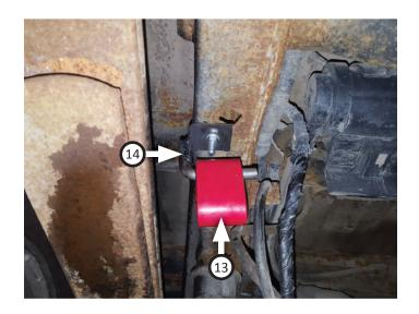
14. Place **clamp (10)** onto **left rear tailpipe (6)** then connect it to left front tailpipe. Insert wire hanger into rubber hanger then tighten clamp just enough to allow for adjustment.
