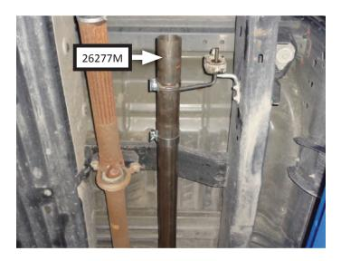
Place 3" clamp (MC300BS) onto muffler (72288-Z) inlet then connect muffler to inlet pipe or extension. Place 2.5" clamps (x2) (MC250BS) onto muffler outlets. Tighten front clamp just enough to allow for adjustment.
