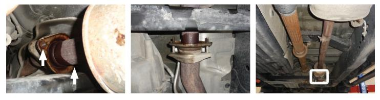
4. Disconnect factory muffler wire hangers (x2) from isolators on vehicle frame.
