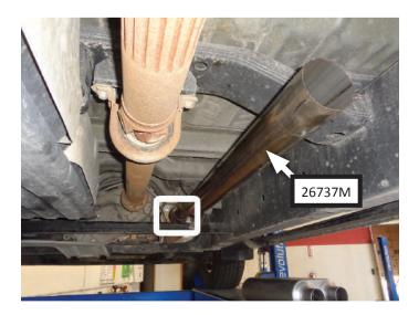
10. Place **3" clamp (MC300BS)** and **front clamp hanger assembly (490HA)** onto **extension pipe (26277M)**. Hang assembly onto vehicle frame and connect to inlet pipe.
