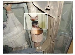
6. Remove remaining muffler assembly from vehicle. Release tab and remove factory clamp from pipe inlet. Retain factory clamp for later re-use.
