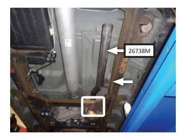
**NOTE:** Complete this step ONLY if your vehicle is a Crew Cab truck with a 6'5" bed. This extension pipe will not be used on Double Cab or Crew Cab-5.5' bed models.
