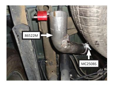
16. Place **2.5"** clamp (MC250BS) onto slip-fit of side exit pipe (86532M) then connect it to left rear tailpipe. Tighten clamp just enough to allow for adjustment.
