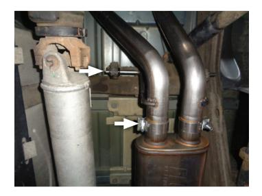
15. Place 2.5" clamp (MC250BS) onto left rear tailpipe (86522M) inlet then connect rear tailpipe to front tailpipe. Tighten clamp just enough to allow for adjustment. Use cable tie (HW505) to secure vent hose and brake lines away from exhaust components.
