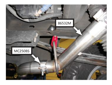
17. Place **2.5"** clamp (MC250BS) onto slip-fit of side exit pipe (86532M) then connect it to right tailpipe. Tighten clamp just enough to allow for adjustment.
