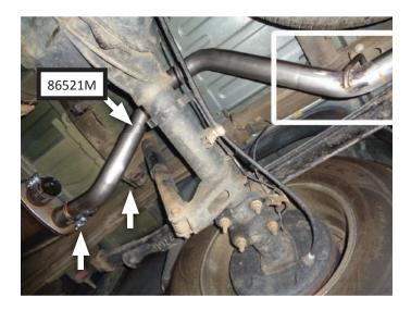
14. Route **left front tailpipe (86520M)** over rear axle then connect it to driver side muffler outlet. Insert wire hanger into stock mount to complete connection. Tighten clamp just enough to allow for adjustment.
