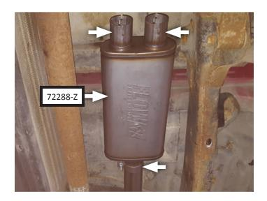
12. Route **right tailpipe (86591M)** and **left front tailpipe (86590M)** over axle and connect them to muffler outlets. Insert wire hangers into isolators then tighten clamps (x2) just enough to allow for adjustment.
