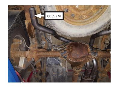
15. Place clamps (x2) (MC250BS) onto slip-fit of side exit pipes (x2) (86593M) then connect them to tailpipes. Tighten clamps just enough to allow for adjustment.
