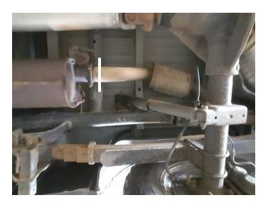
4. Support muffler and disassemble wire hangers from isolators. Remove clamp on slip connection behind cat. converter. Heat or cut slip connection to separate components, then remove muffler portion of exhaust from vehicle.
