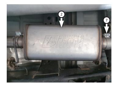
11. Route **tailpipe assembly (3)** over axle then connect it to muffler. Insert wire hangers into factory isolators then tighten clamp just enough to allow for adjustment.
