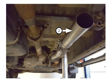
11. Place front hanger (8) onto muffler (3) then connect it to inlet/extension. Insert hanger into isolator and tighten clamp just enough to allow for adjustment.
