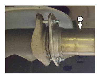
10. For applicable vehicles, place clamp (6) onto extension pipe (2) and connect it to inlet. Inlet pipe should be offset toward frame of vehicle.
