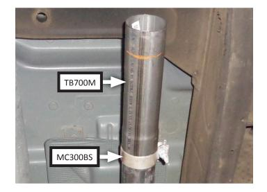
8. Place clamps (x2) (MC300BS) onto muffler (71249-Z) and connect it to inlet pipe. Tighten clamp just enough to allow for adjustment.
