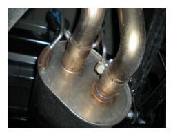
2) Loosen the two clamps at the back of the muffler and carefully slide the tailpipes toward the rear to remove from the muffler. Allow the pipes to hang until installation of the Flowmaster muffler.
