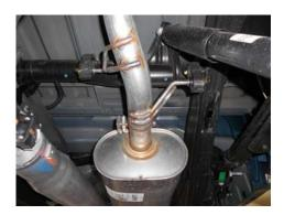
2) Support the muffler with a stand. Using a hacksaw or sawsall, cut the stock tailpipe off just behind the muffler. Separate the wire hangers on the tailpipe from the rubber mounts on the vehicle and remove the tailpipe from the vehicle. This step is not mandatory but makes removal easier.
