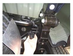
5) Remove the 3 factory rubber exhaust isolators from the mounts on the vehicle, two just forward of the rear axle and one at the rear of the vehicle.
