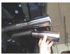
8) Place the **#ST439** stainless tips onto the ends of the tailpipe assembly and adjust to the desired position. Tighten the pinch clamps on the tips enough to hold in position.
