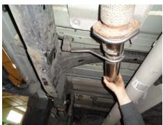
3) Place clamp hanger assembly **502HA** over the back of the inlet pipe and connect to the rubber mount on the vehicle.
