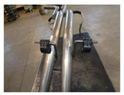
6) Place the rubber isolators removed in the previous step onto the 3 wire hangers of tailpipe assembly **86486M**.
