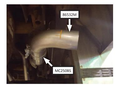
18. Place **tips (x2) (ST507B)** onto side exit pipes. Tighten clamp just enough to allow for adjustment.
