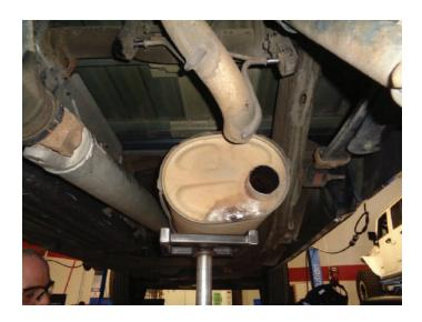
4. Apply lubricant to factory isolators (x3) shown then remove factory wire hangers (x3) from isolators. Remove trimmed factory tailpipe from vehicle.
