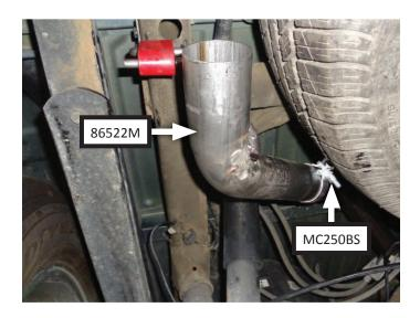
Place 2.5" clamp (MC250BS) onto slip-fit of side exit pipe (86532M). Connect rear exit pipe onto left rear tailpipe. Tighten clamp just enough to allow for adjustment.
