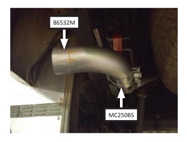
17. Place 2.5" clamp (MC250BS) onto slip-fit of side exit pipe (86532M). Connect rear exit pipe onto right tailpipe. Tighten clamp just enough to allow for adjustment.
