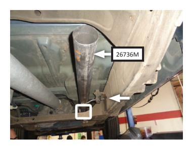
**NOTE:** Complete this step ONLY if your vehicle is a Crew Cab truck with a 6'5" bed. This extension pipe will not be used on Double Cab or Crew Cab-5.5' bed models.
