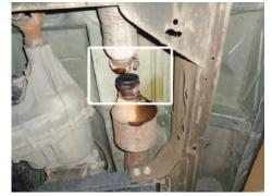
6. Remove remaining muffler assembly from vehicle. Release tab and remove factory clamp from pipe inlet. Retain factory clamp for later re-use.
