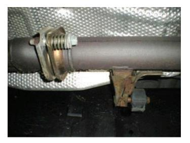
5. Separate hangers (x4) on muffler and front pipe assembly from rubber mounts on vehicle; then remove assembly from vehicle.
