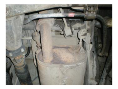
4. Remove factory spring loaded bolts (x2) at inlet pipe flange connection and set aside. Retain bolts and springs for later use.
