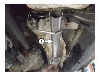
9. Place **clamps (x2) (5)** onto **FFX muffler (2)** then connect it to inlet pipe. Tighten front clamp just enough to allow for adjustment.
