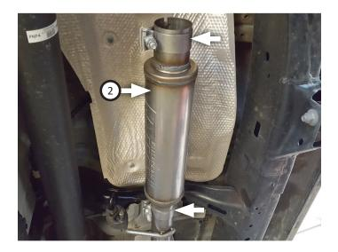
Route overaxle assembly (3) over axle and connect it to muffler then insert wire hangers in mounts. Place clamp (5) onto exit pipe assembly (4) and connect it to overaxle pipe. Tighten clamps enough for adjustment.
