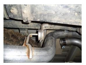
2) Loosen the two clamps connecting the tailpipes to the muffler at the over-axle slip-fit connections. Then unbolt the forward hanger mount on each tailpipe from the frame. Leave the hanger mounts connected to the tailpipes.
