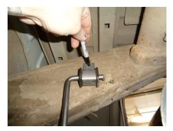
6) Adjust the exit pipe so that the tips are the desired distance from the body, then rotate the **HA572** hanger so that it lays flat against the inside of the vehicle frame and use a center punch to mark the center of the two holes on the frame. Rotate the hanger out of the way and drill each mark using a ¼" drill bit. Use the two 5/16" thread cutting bolts to secure the hanger to the frame. Tighten securely.
