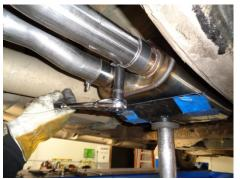
5) Place a supplied 2-1/2" clamp onto each muffler outlet. Place the exit pipe assembly **#86465M** up into position and slide into both muffler outlets approximately 2". Use a stand to support the outer end of the assembly. Tighten the clamps just enough to hold in position.
