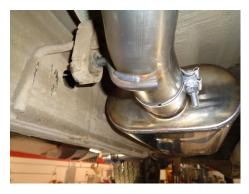
3) Place a supplied 3" clamp over the inlet of the muffler, then slide the muffler onto the back of the inlet pipe. Use a stand to support the muffler. Tighten the clamp enough to hold in position.
