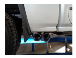
7) Adjust the position of all pipes and muffler to provide a satisfactory fit. A minimum 3/4" clearance around all parts of the system must be maintained; while also keeping suspension travel and vibration in mind.
