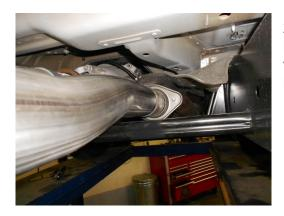
2) Place the inlet pipe onto the back of the existing OEM head pipe and fasten using the 3/8" x 2.00" bolts, nuts and washers provided in the hardware kit. Tighten just enough to hold in place, but still allow for adjustment.
