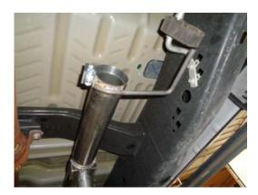
3) Slide the inlet hanger **#490HA** over the back of the inlet pipe and insert the hanger into the factory rubber mount. Do not tighten this clamp yet. **Note:** See step 4 if the frame hanger does not line up with clamp hanger 490HA.
