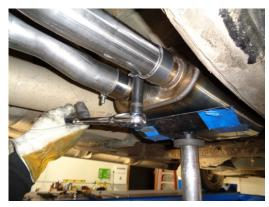
7) Place a supplied 2-1/2" clamp onto each muffler outlet. Place the exit pipe assembly **#86467M** up into position and slide into both muffler outlets approximately 2". Use a stand to support the outer end of the assembly. Tighten the clamps just enough to hold in position.
