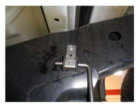
8) Adjust the exit pipe so that the tips are the desired distance from the body, then rotate the **HA572** hanger so that it lays flat against the inside of the vehicle frame and use a center punch to mark the center of the two holes on the frame. Rotate the hanger out of the way and drill each mark using a ½" drill bit. Use the two 5/16" thread cutting bolts to secure the hanger to the frame. Tighten securely.
