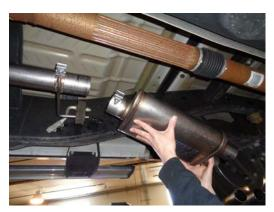
5) If required, place the extension pipe **#26277M** onto the back of the inlet pipe. Then place a supplied 3" clamp onto the muffler inlet and slide the muffler onto the inlet pipe approximately 1.75" and support with a stand. Level the muffler and tighten the clamp at the inlet enough to hold, but still allow for adjustment.
