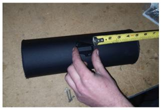
Place MAF adapter onto tube and center it. Make sure slot aligns with center line of tube. Adapter should sit perfectly flat.
