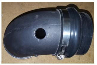
1. Remove IAT sensor from your vehicle, then use sensor to mark and drill an appropriate sized hole in your new intake system.
