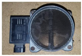
This style MAF is housed and will have to be integrated into your tubing assembly. Start by uninstalling housing from vehicle.
