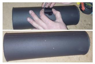
4. Mark mounting hole through MAF adapter onto tube.
