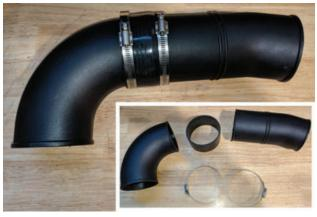
6. Construct your route from throttle body to air filter location. Each tube connects using a coupler and two clamps as shown. Remember to integrate MAF sensor and Intake Air Temperature (IAT) sensor as well.
