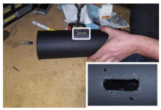
7. Disassemble parts from tube then drill marked slot for MAF Sensor. You can oversize your drill up to an 1/2" so your MAF Sensor slides in and out easily. Deburr and smooth drilled edges.
