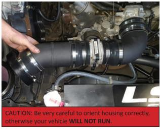
3. Install housing into intake assembly. For most effective reading, center it between straight tubes.
