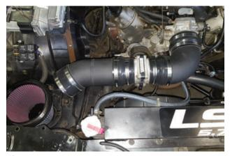
1. Install air intake kit onto throttle body, routed over to air filter location.
