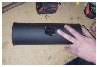
8. Apply RTV to MAF adapter and install it onto tube using (x2 ea) screws to locate it properly. Use locknuts (24) to secure adapter in place then wait for RTV to set (approximately 1 hour).
