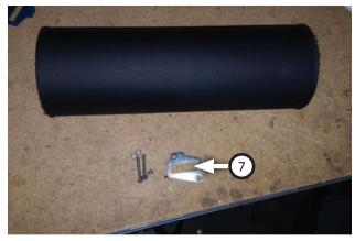
2. Gather **MAF adapter (7)** and select tube in which you are going to install MAF sensor.
