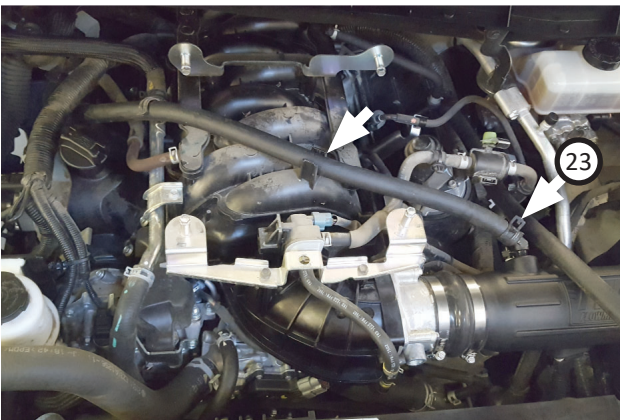
25. Route fuel hose over engine to 45° hose barb. Mark hose where it can press fully onto barb, then cut it at mark. Connect hose to barb and secure it using pinch clamp (23).
