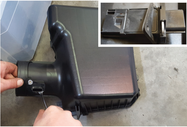
18. Remove and retain MAF sensor from factory airbox cover.
