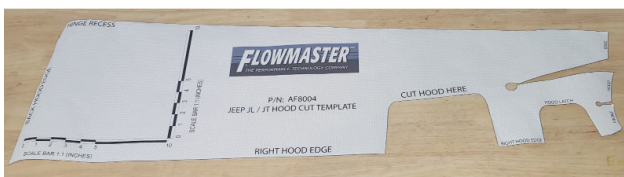
38. Carefully cut out paper hood cut template from kit. Be as precise as possible.
