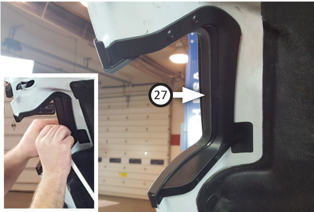
60. Apply foam strip (27) to inside edge of hood adapter gasket. Work from one end, pressing it on fully then cut strip to length so it works as a seal.
