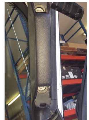
23. Release cover from base of A pillar then remove bolt covers from passenger grab handle on A pillar.
