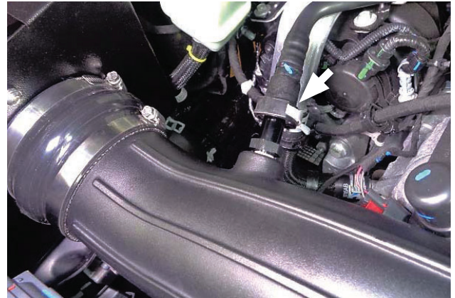
33. Connect PCV line to quick connect fitting, then make sure all connections are secure.
