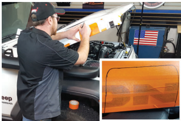
43. Mark hood (tape) around edge of template cutout then remove template from vehicle.
