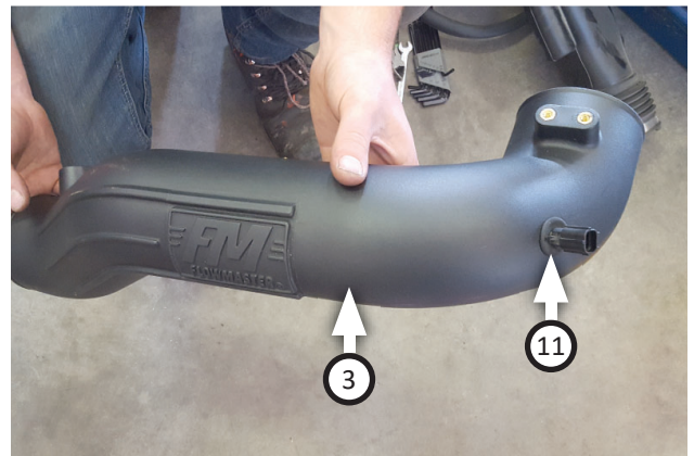
NOTE: Lubricate grommet as needed to ease install. 16. Fit grommet (11) into intake tube (3) then insert IAT sensor (from previous step) into it as shown.
