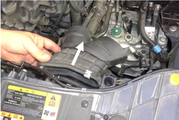
13. Pull straight back on the inlet air duct to remove it from the vehicle.
