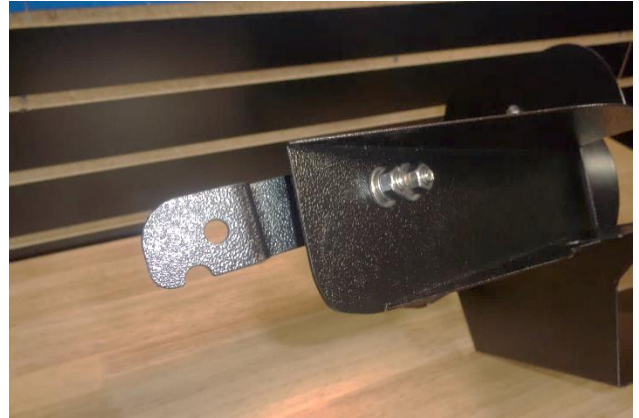
22. Attach bracket (10) to the inlet air duct using 1/4-20 screws (9) (on the bracket side), and flat washers (8), lock washers (7) and nuts (6) (on the duct side).
