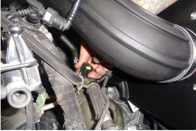
37. On the bottom of the inlet tube, connect the air temp sensor plug to the sensor and check the plug for security.
