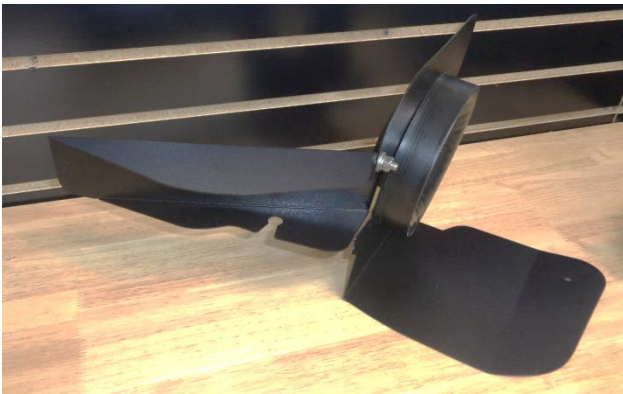
20. Assemble the inlet air duct (5) to the heat shield using a 1/4-20 screw (9) (on the duct side), and a flat washer (8), lock washer (7) and nut (6) (on the heat shield side).
