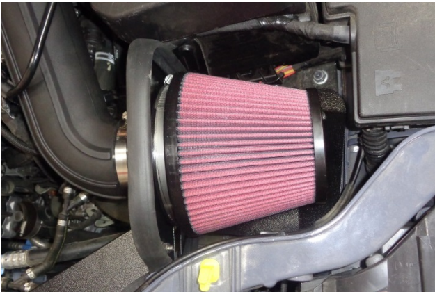
38. Place clamp (2) on air filter (1), install the filter on the filter adapter, and tighten the clamp.
