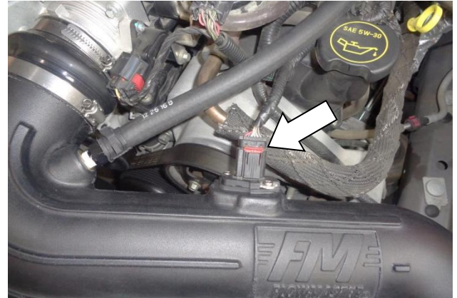
28. Reconnect the MAF sensor plug to the sensor, close the locking tab, and verify the connection is secure.
