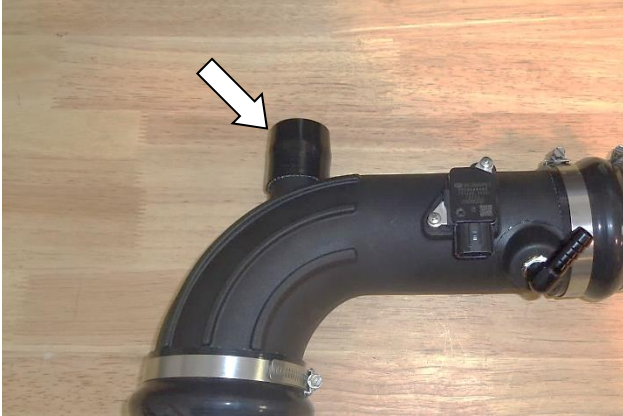
19. Push the small coupler (16) all the way onto the intake tube resonator port.
